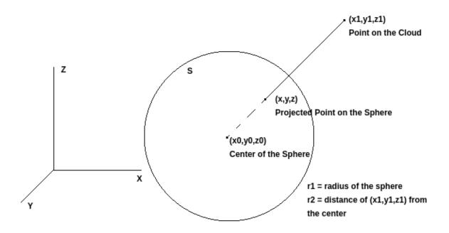
The figure above shows the spherical projection of a point onto the surface of a sphere with radius  $r_1$  and with its center at the point( $x_0$ ,  $y_0$ ,  $z_0$ ). Such a sphere can be represented by the following equation
