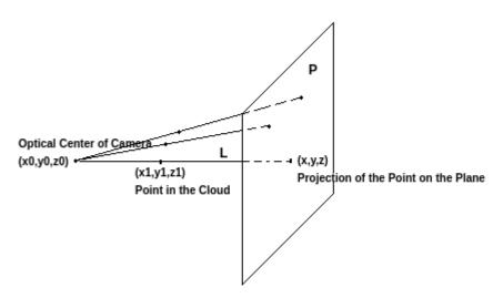
The above demonstration shows the perspective transform of a set of points onto the plane P from the optical center of the camera, with arbitrary co-ordinates  $(x_0, y_0, z_0)$ . We can see that the projection (x, y, z) of a point  $(x_1, y_1, z_1)$  on the plane P is nothing but the point of intersection between the said plane and a line L passing through the optical center and the given point in the cloud.
